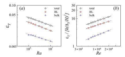
**FIG. 8**. (a) Thermal energy dissipation rates as a function of Ra; (b) normalized thermal energy dissipation rates as a function of Re. The lines are the power-law fits to the corresponding data.
