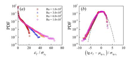
**FIG. 5.** (a) Probability density functions (PDFs) of the thermal energy dissipation rate  $\varepsilon_T(\mathbf{x},\ t)$ , and (b) PDFs of the normalized logarithmic thermal energy dissipation rate  $\log \varepsilon_T(\mathbf{x},\ t)$  obtained over the whole cell; the dotted-dashed line represents a log-normal distribution.
