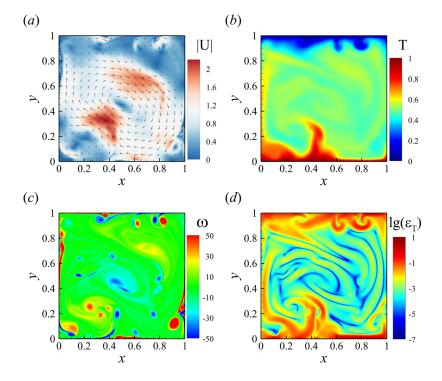
**FIG. 1**. A typical snapshot of an instantaneous flow field (a) and its corresponding temperature field (b), vorticity field (c), and logarithmic thermal energy dissipation rate field (d) for  $Ra = 10^7$  and Pr = 0.025.
