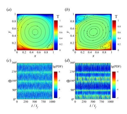
**FIG. 2.** [(a) and (b)] Time-averaged temperature fields and streamlines, [(c) and (d)] time evolution (from left to right) of the probability density functions (PDFs) of the instantaneous velocity vector orientation  $\theta$  for Pr = 0.025 [(a) and (c)] and Pr = 5.3 [(b) and (d)] at  $Ra = 10^7$ .
