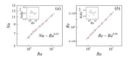
**FIG. 3**. (a) Nusselt number and (b) Reynolds number as functions of Rayleigh number for Pr = 0.025. The solid lines are the power-law fits to the data. The insets are the compensated plots of the data shown in (a) and (b), respectively.
