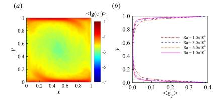
**FIG. 6.** (a) Time-averaged logarithmic thermal energy dissipation field obtained at  $Ra = 10^7$  and Pr = 0.025, and (b) vertical profiles of horizontal- and time-averaged thermal energy dissipation rates for Pr = 0.025 and various Ra.
